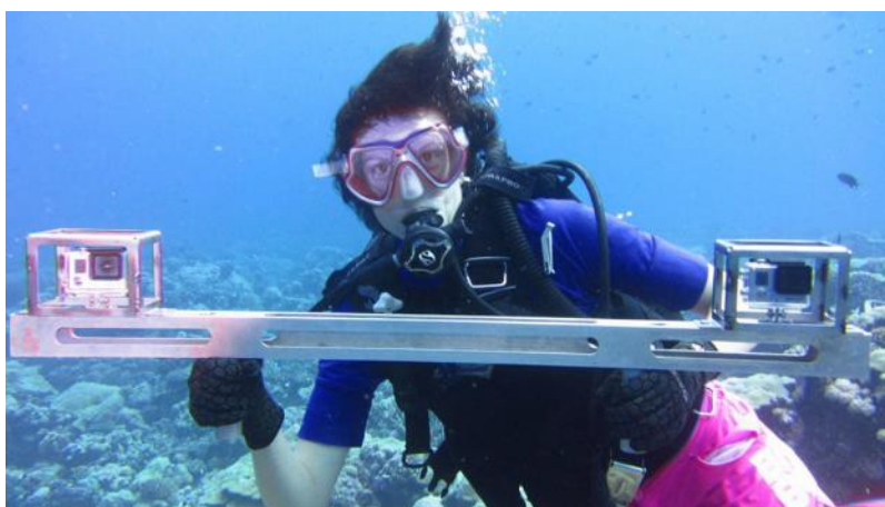
Figure 4: Operation of stereo-DOVS rig with mounted GoPros.
