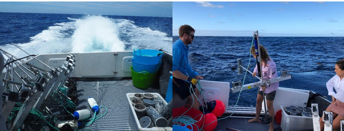
**Mid-water baited remote underwater video systems(BRUVS) racked up *en route* to sampling location (left) and deployment of the BRUVS (right) at the Eastern Recherche Marine Park**
